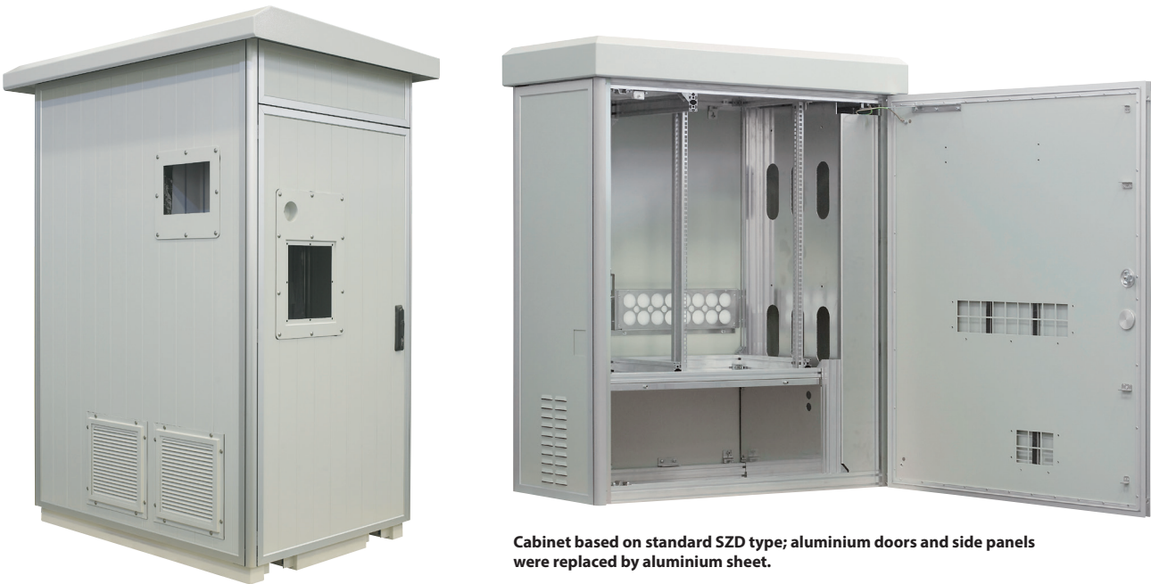
Cabinet for battery charger
